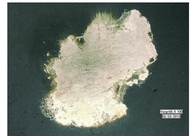
Self-healing event in typical metalized film
