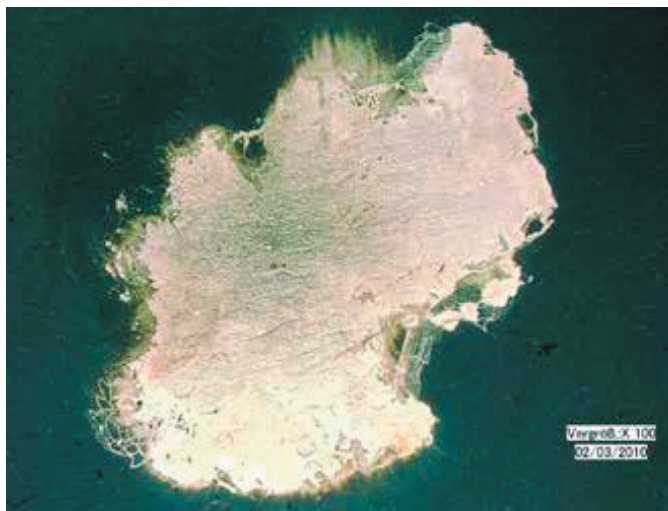
Self-healing event in typical metallized film
