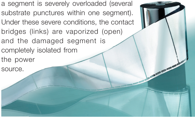
FRAKO Segmented, self-healing metallized film
